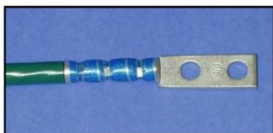
Figure 14. Example of a barrel with three crimps
